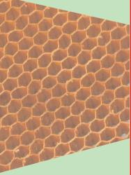
Nomex<sup>®</sup> honeycomb was developed with the advent of the wide-body commercial airplane for use in flooring, bulkheads, dividers, galley structures and lavatories. General Veneer Manufacturing Co. was among the first to use it in production. Nomex® core offers high impact resistance and compressive properties and performs superbly on the food cart roller test.
